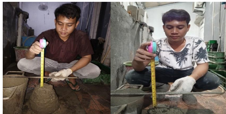
Gambar 8 uji slump test
